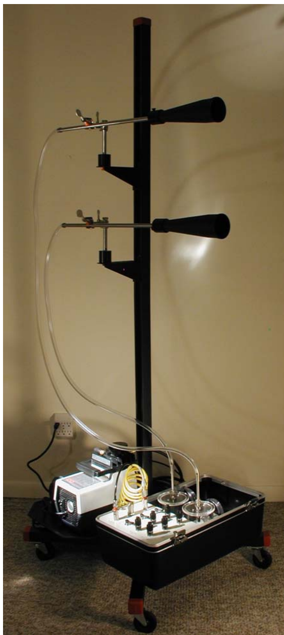
SAI™ Rolling Stand w/ Wands, Bubble Generator and Auxiliary Air Helium Supply
